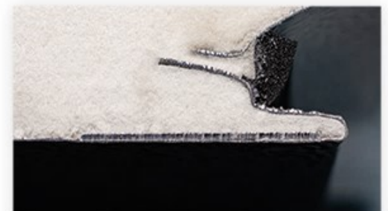
Inside 1.0mm steel plate
